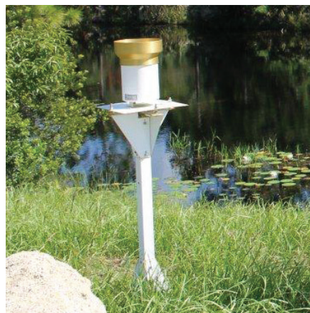
Rainfall tipping bucket with mounting stand
