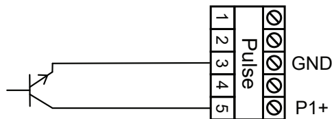
Figure 5D: Open collector NPN transistor
