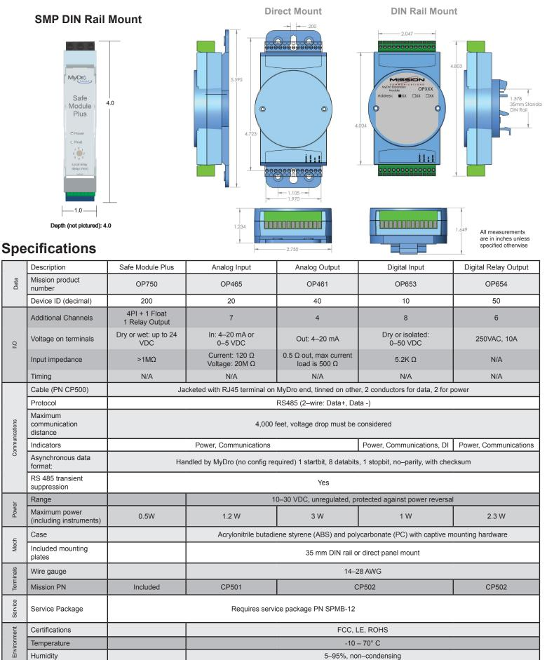
\*The MyDro RTU can source up to 3W over the communications cable, and share the battery capacity with expansion modules and instruments when loss of AC power occurs. The ampacity of the standard 5Ahr yields 60Whr. Consider upgrading the backup battery (PW427) for longer use when no main power is available.
