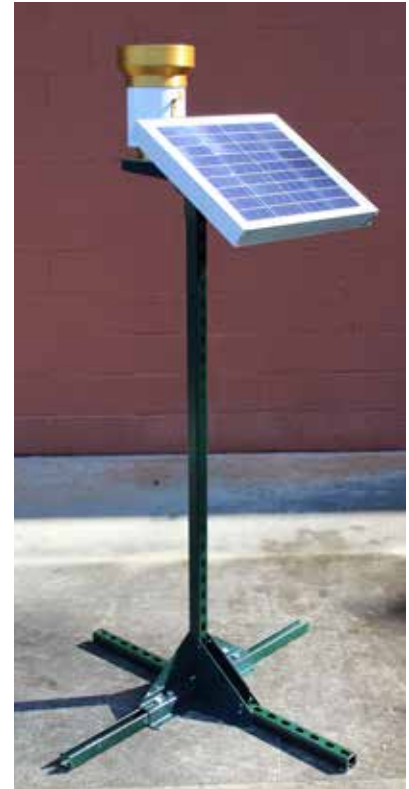
Universal stand with rain tipping bucket and solar panel
